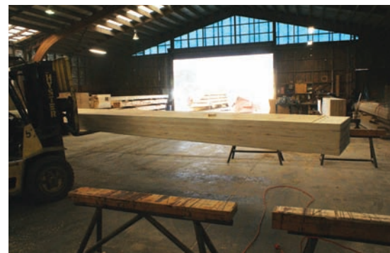
Figure 18 Fabricated LVL column for installation at new Nelson Pine dispatch hall
