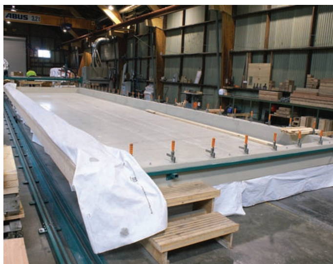
Figure 19 Cross Laminated Timber press, XLam factory
