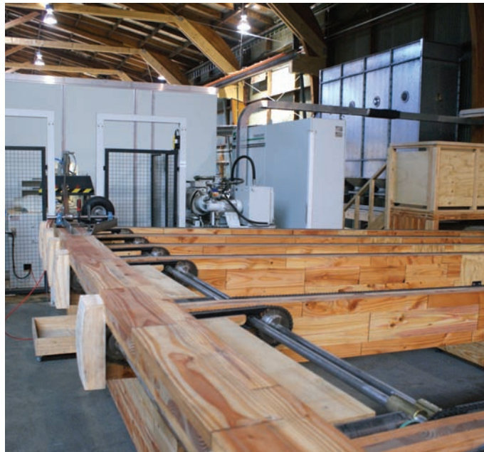
Figure 20 Boards come out of finger jointing machine onto this storage platform, itself constructed from CLT
